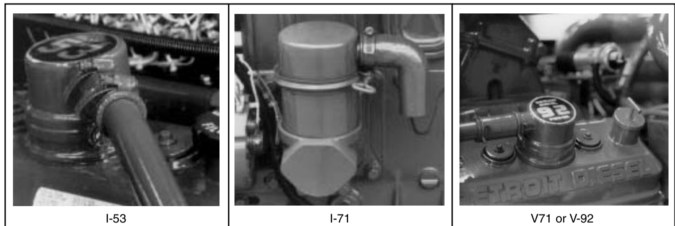
Figure 2 - Crankcase Ventilation
